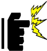
Always ground yourself to remove any static charge before touching the CPU card. The electronic devices are very sensitive to static electricity. For safety concerns, please use a grounding wrist strap all the time. Place all electronic components in a static-dissipative surface or static-shielded bag when they are outside of the chassis.
