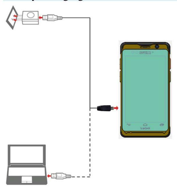
Method 1: Using the supplied power adapter and USB cable to connect the phone to a power outlet.
