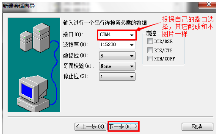
Figure 2.7 CRT Serial Port Setting
