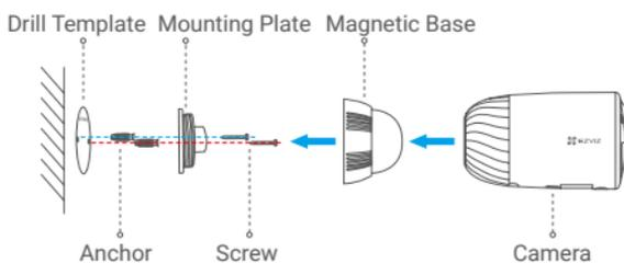
Fig.1 Mount by Magnetic Base
