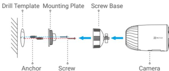
Fig.2 Mount by Screw Base
