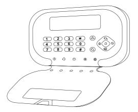
DS-PK00/PK00M/-LCD/LED series LCD/LED alarm keypad are used for connecting to the security control panel. It implements operations on the security control panel through programming and prompts alarm with the indicators and audio alert.
