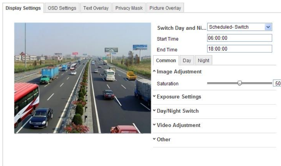
Figure 6-37 Day/Night Scheduled-Switch Configuration Interface
