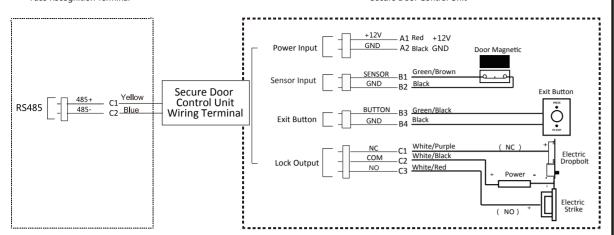
Note: The secure door control unit should connect to an external power supply separately. The suggested external power supply is 12 V, 0.5 A.
