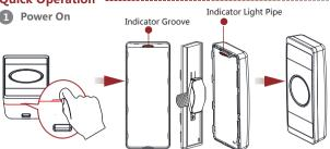
Dig the groove to disassemble the device. Remove the front and rear panel. Remove the insulating strip to power on the device.
