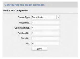
Figure 4-1 Configure Indoor Station No.
