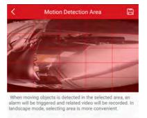
Figure 3-5 Draw Motion Detection Area
