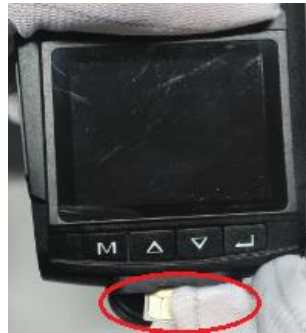
Figure 1. 3 Insert SIM Card
