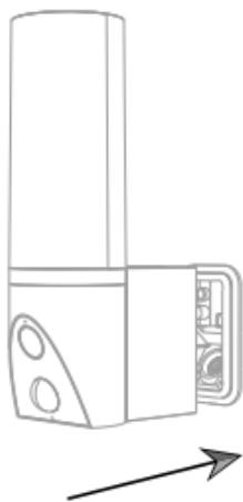
Install the camera into the bracket along the direction of the bracket.
