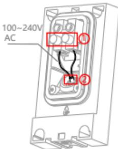
1. Loosen the screws of ① and connect the power cable to the terminal. And then tighten the screws of ①.
