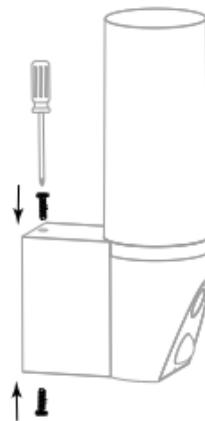
After the camera is installed in the bracket, fix them with screws.
