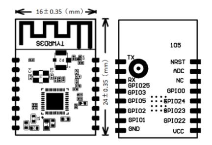
Figure 1 TYWRD3S front and back views
