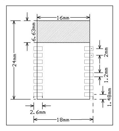
Figure 5 TYWRD3S encapsulation on the PCB
