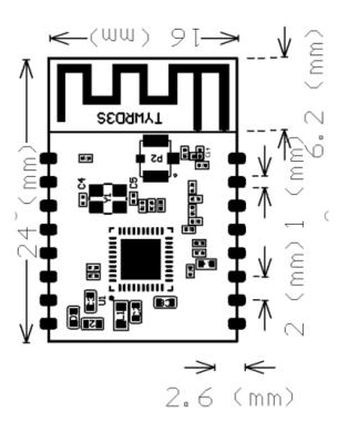
Figure 2 TYWRD3S mechanical dimensions
