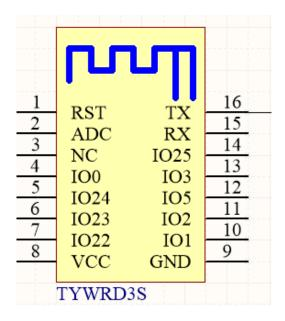
Figure 4 TYWRD3S schematic diagram and pin connection
