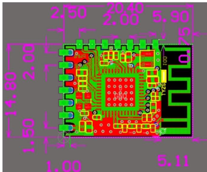
Figure3: The TYZS5mechanical dimensional drawing
