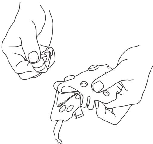
4. One hand holds the Cover, while the other press the block into the block slot.
