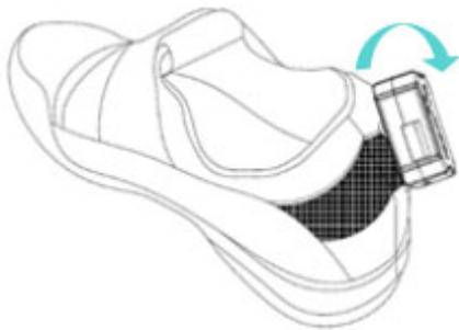
Finish the installation of the KATVR-Foot Sensor.
