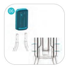
Place the back-support plate on top of the rods. Fix it with the screws and gaskets (Items No. 12 and 13). Temporarily do not tighten them completely - only turn each of them 3 times.
