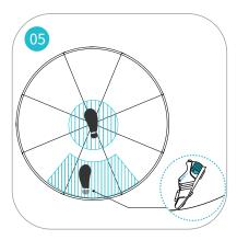
To trigger movement backward, place one of your feet at the center of the platform and keep the other one at the back edge with heel up.
