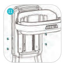
Insert the plugs into the openings on the sides of the device.
