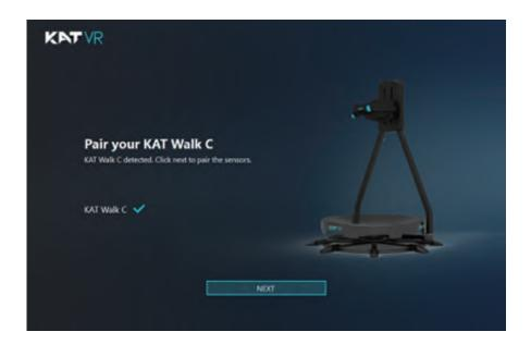
Click "NEXT" and use the gray cable of the tiple-ended micro USB wire from the KAT Walk C sensor kit to connect the foot sensors to your PC. Follow the software instructions and click "FINISH" to complete the sensor pairing.
