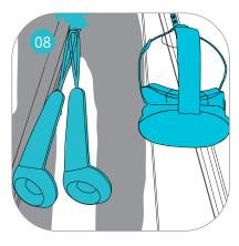
Pick the headset and controllers from the storage hooks at the back of the device.
