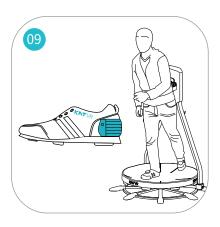
Pull up the anti-slip protection straps from the shoe heel.Practice walking for a few minutes until you get used to the simulative gait.
