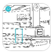
Cut the wire tie on the bottom of the base.
