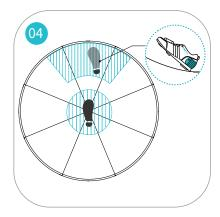
To trigger continuous movement forward without walking (cruise mode), place one of your feet at the center of the platform and keep the other one at its front edge with toes up.
