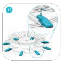
Install the eight base stabilizing feet (List: No.14, No.15).
