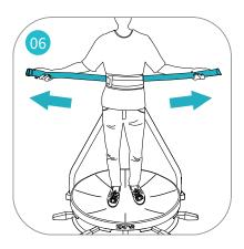
In the same order from left to right, fasten the belts on your waist making sure the Velcro is well aligned. Press the end to ensure it is fastened firmly (DANGER: Fastening the belts too loose or diagonally may cause safety hazards, walking direction deviation etc.)
