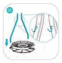
Align the support rod with the rod opening at the side of the platform and insert it.
