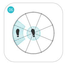
To trigger strafing left, place your right foot at the center of the platform and keep the left one at the left edge with toes directed forward and heel up. Wrong toe direction may cause movement deviations.
