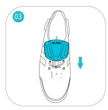
Push the sensor slot into the shoe socket from the top toward the toes side. The LED lights should be facing the toes.
