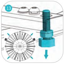
Level the rotational beam through adjustment of 4 screws at the edge of the structure. Tighten or loosen them until the beam rotates smoothly without deviations.
