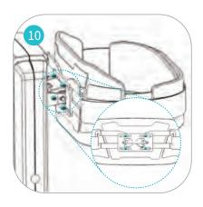
Install the screws. Note: Misaligned or loosen screws will affect the operation of the device. For more information about the installation method, please refer to the complete user's manual.
