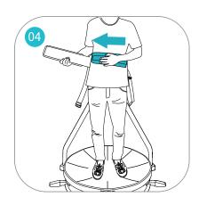
Stretch the left belt and pull it onto your waist. Stretch the right belt and paste it on the left one, making sure the Velcro is well aligned. Press the end of the belt to ensure it is fastened firmly (DANGER: Fastening the belts too loose or diagonally may cause safety hazards, walking direction deviation etc.)
