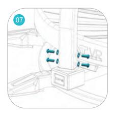
Install the screws and gaskets at the bottom of the rods (Items No.14 and 15). Note:Tighten them well to avoid safety hazards.
