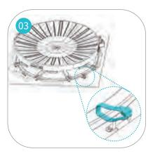
Cut the cable tie holding the base.
