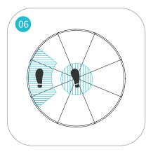
To trigger strafing left, place your right foot at the center of the platform and keep the left one at the left edge with toes directed forward and heel up. Wrong toe direction may cause movement deviations.
