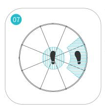
To trigger strafing right, place your left foot at the center of the platform and keep the right one at the left edge with toes directed forward and heel up. Wrong toe direction may cause movement deviations.
