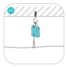
Hang the wire pulley onto the hook.
