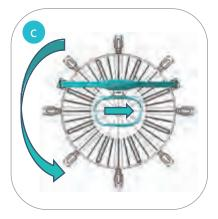
If the beam tends to continuously turn counterclockwise, please move the waist harness slightly to the right.
