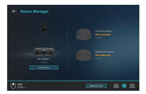
The device manager page shows the status of each sensor and the SN of the device. Through this page, you can initiate the sensor pairing process
