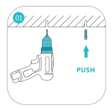
Drill a hole in the ceiling about 1m (horizontally) away from the center of the treadmill. Place the expansion screw sleeve into the hole.
