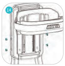
If the beam continues to return to the same position, lower the opposite side of the platform by adjusting the corresponding screw (turn it right). Once leveled, tighten the upper nuts.
