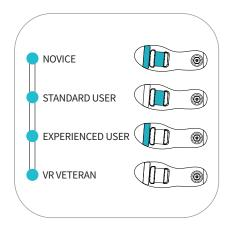
The KAT Shoes 2 have two anti-friction stripes on the shoe sole and offer four adjustable levels of friction (as pictured). Their purpose is to let the user adjust the kinetic friction force between the shoe sole and the platform to own preferences. When using the device for the first time, it is recommended to keep the friction force on the Novice level, and gradually adjust it as the user proficiency in using the device grows.
