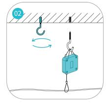
Mount the hook into the expansion screw sleeve, tighten,
