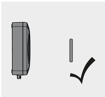
If the data carrier antenna is aligned vertically to the read/write head, this will only result in poor performance and a minimum read range. Vertical alignment should therefore be avoided.
