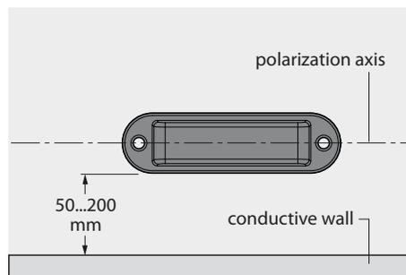
A minimum distance to two conductive walls must be observed for the data carriers. This is 50...200 mm parallel and vertical to the polarization axis.
