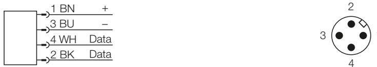
The .../S2501 cables have the following wiring diagram (“Figure 30: Wiring diagram for .../S2501 cables”).
