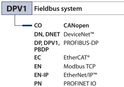
exception: BL67-GW-EN can be used for Modbus TCP and EtherNet/IP™
