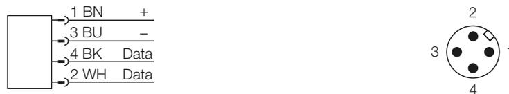
The .../S2503 cables have the following wiring diagram (“Figure 31: Wiring diagram for .../S2503 cables”).
