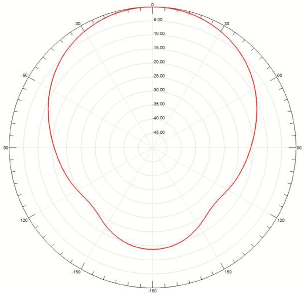
**A.1.3 Elevation section, horizontal polarization**
