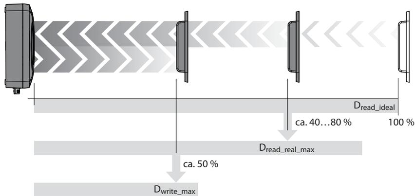
Reserve capacity must be included in planning, not only with regard to the possible radio range, but also with regard to time available for accessing the data carrier on the fly within a time window.
