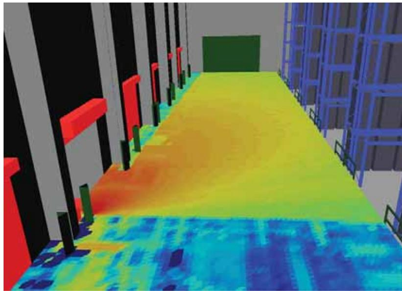
All the essential physical factors involved in the propagation of radio waves are taken into account. These include for example: Attenuation characteristics in air and other media (obstacles), reflection and transmission properties on objects of different materials, polarization characteristics, antenna characteristics and gain of read/write units and data carriers.
