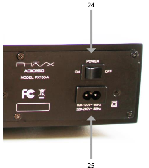
Fig. 10 ADIO150 Rear Panel AC MAINS Connector
