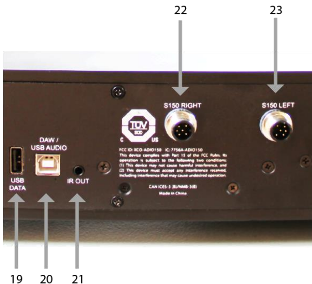
Fig.9 The ADIO150's Rear Panel USB/DAW and Speaker Connectors
