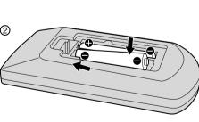
■ To close the cover, insert the protrusion at the bottom of the cover into the notch on the remote control and then push down the top of the cover until a click is heard
