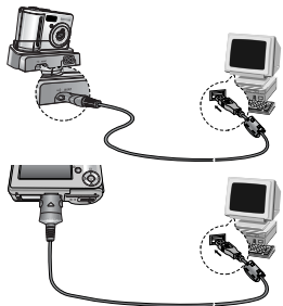
[Using the USB cable with Cradle]
