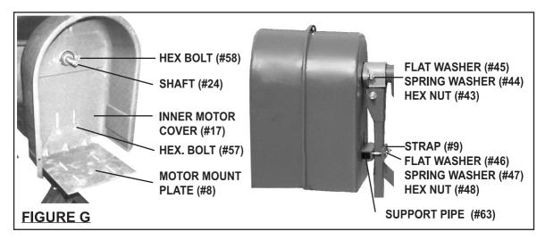
17. Attach the Motor Mount Plate (#8) to the Inner Motor Cover (#17) using the Hex. Bolt (#57), Flat Washer (#46), Spring Washer (#47) Hex. Nut (#48), and Strap (#9). Tighten sufficiently to hold in place. See photo above.
