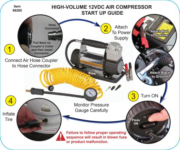
Turn unit on *before* connecting to tire valve. This will prevent blowing of fuse.
