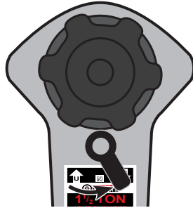
Figure I: 66106/96482 Selector Lever “D” / Down Position
