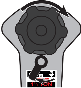
Figure H: 66106/96482 Selector Lever and Brake Knob “U” / Up Position
