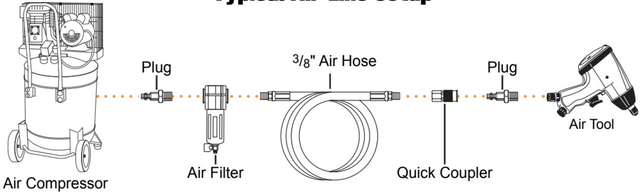
Thread seal tape is recommended for all threaded connections.
