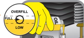
**3** Fill Compressor Pump with oil. Do not overfill. (Oil sold separately.)
