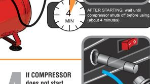
does not start, check FUSE, replace if needed.
