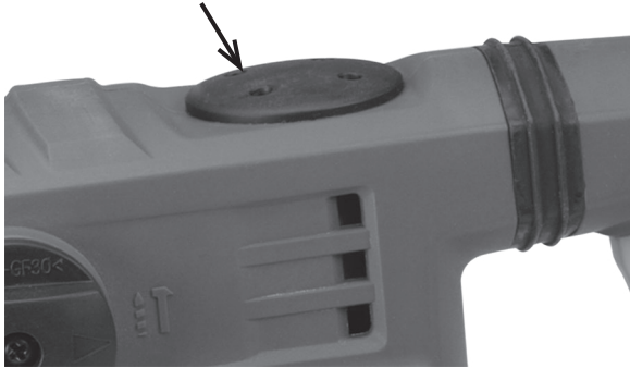
Figure E: Grease Port
