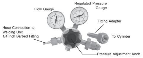
Regulators attached to the cylinder valve reduce high cylinder pressures to a suitable low working pressure for welding applications. Always set to the recommended pressure for the welding operation to be performed.
