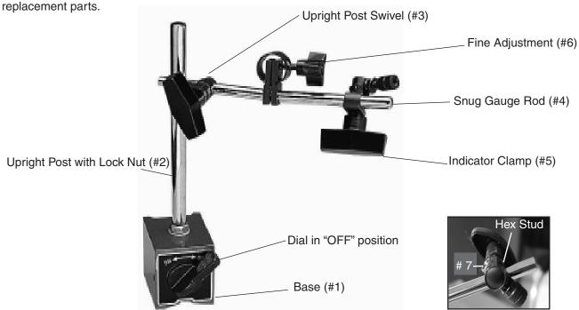
Note: Part# 7 (5/16" Adjustment Bushing) fits into part# 5. It will allows you to clamp 5/16" stem dial indicators. Without the bushing it will clamp 3/8" stem dial indicators. The bushing is held in place with a small hex stud.
