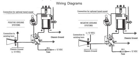
Always use vehicle terminal type connectors (not supplied) on all connections. Never wrap wires around terminals as they could fall off. Connect terminal #30 on the Electric Relay (6) to a 30A fused circuit.
