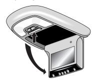
Press the release button, as shown. The screen lowers and the RSE system powers on automatically.
