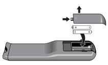
Battery life is approximately 50 hours depending on how often the remote is used. Use two size-AAA batteries. Replace both batteries at the same time.
