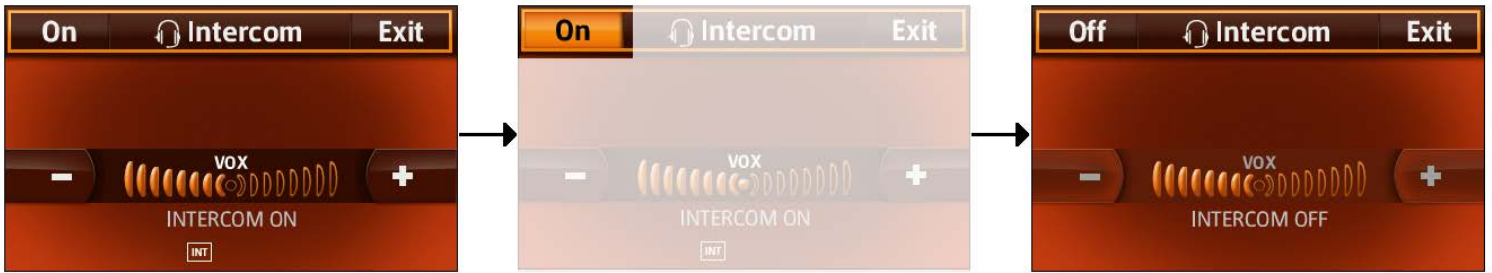
Figure 17. Turning Intercom Off
