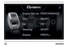
"Engine Set Up": PERFORMANCE (greater response + Overboost to maximise the torque level - for versions/markets, where provided)  "ESC": SPORT (intervention thresholds for more enjoyable, sporty driving, guaranteeing stability in case control of the car is lost.
