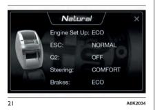
□ "Engine Set Up": ECO (standard response)
