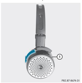
The battery compartment is located on the left headphone. The cordless headphones require 2 type AAA, 1.5 V batteries.
