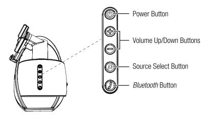
**Power button:** Press this button to turn the JBL OnBeat Xtreme on. The Power Button LED will glow white. When the system is on, press this button to place the system in the sleep mode. The LED will glow amber.
