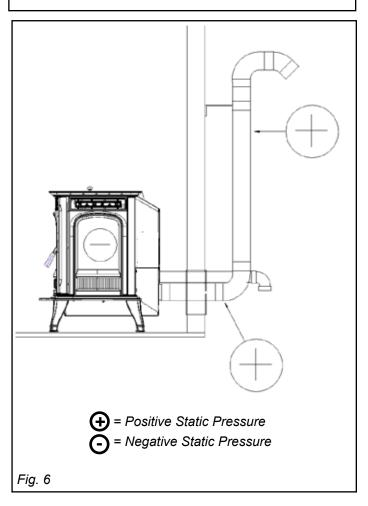
INSTALL VENT AT CLEARANCES SPECIFIED BY THE VENT MANUFACTURER.
