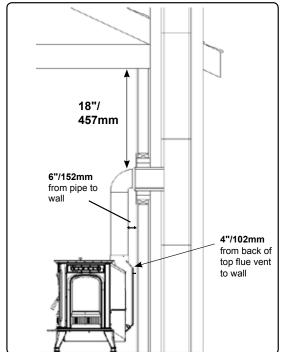
Fig. 5: Optional Top Vent Pipe Clearances
