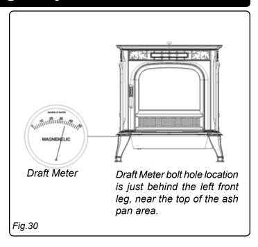
A simple draft test should be performed after completing the flue pipe installation. To record the results for future reference:
