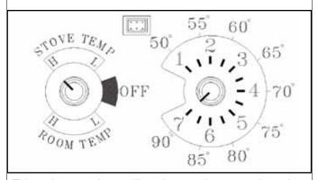
This setting, see above, will produce continuous maximum heat output with the distribution blower at full speed.
