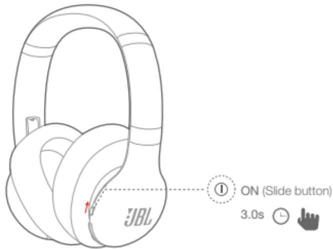
2. If connecting for the first time, the headphone will enter the pairing mode automatically after it is powered on
