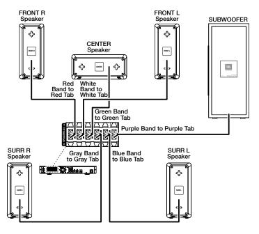
IMPORTANT: Make sure the (+) and (-) bare wires do not touch each other or any metal object on the receiver's rear panel. Touching wires can cause a short circuit that can damage the BD100 receiver.
