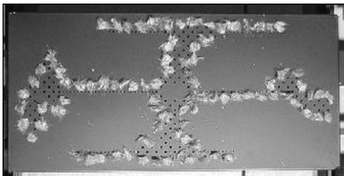
Figure 14. Placement of the Ember Material
