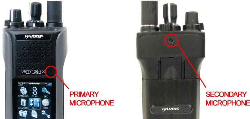
Figure 4-6: Without a Speaker Microphone Attached
