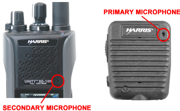
Figure 4-7: With a Speaker Microphone Attached
