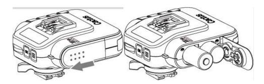
Open the battery door by pushing it backward. Flip open the latch and insert two AA batteries using the correct polarities. Then close the battery door by pushing it to the front.
