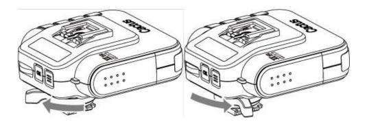
To mount the V6 IIs on a camera's hot shoe mount:
