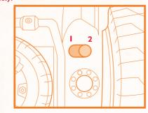
TROUBLESHOOTING: If the toy doesn't respond, make sure the vehicle and controller are on the same channel. If the vehicle and controller are on the same channel and the vehicle still doesn't respond, replace the batteries.
