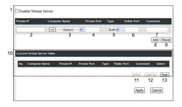
Enable Virtual Check this box to enable virtual server,
