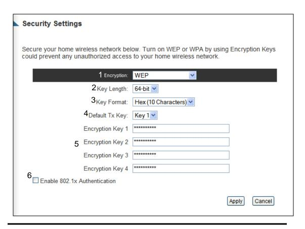
Key Length (2): There are two types of WEP key length: 64-bit and 128-bit.
