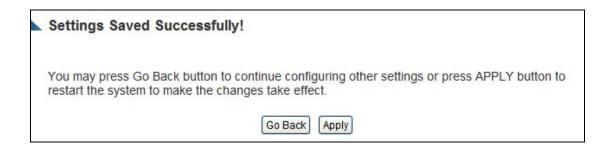
Press "Go Back" to save the settings and go back to the web management interface; press "Apply" to save the settings made and restart the Smart Dish Repeater. The settings will take effect after it reboots.
