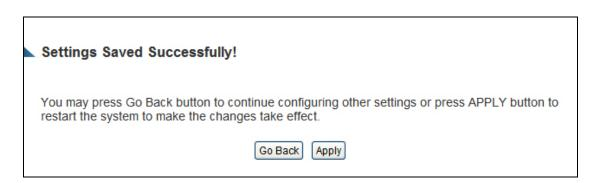
Press "Go Back" to save the settings and go back to the web management interface; press "Apply" to save the settings made and restart the Smart Dish Repeater. The settings will take effect after it reboots.
