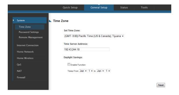
Please click "System" tab in menu on the left of web management interface, then click on "Time Zone". Please select the correct time zone from the drop-down list, and input the IP address or host name of time server. If you want to enable daylight savings time settings, please check "Enable Function" box, and set the duration of daylight setting. When you finish, click "Apply". You'll see the following message displayed on web browser:
