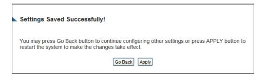
Press "Go Back" to save the settings and go back to the web management interface; press "Apply" to save the settings made and restart the Smart Dish Repeater. The settings will take effect after it reboots.
