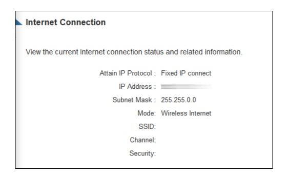
This information will vary depending on the connection status and the type of internet connection that you are using. It will provide IP information, the Internet connection mode (i.e. wired or wireless) as well as the details of a wireless connection.
