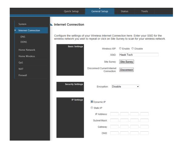
You may manually enter the SSID of the wireless network you plan on connecting to or you can click "Site Survey" to have the web interface scan for local networks in your vicinity. (See Site Survey Menu below)
