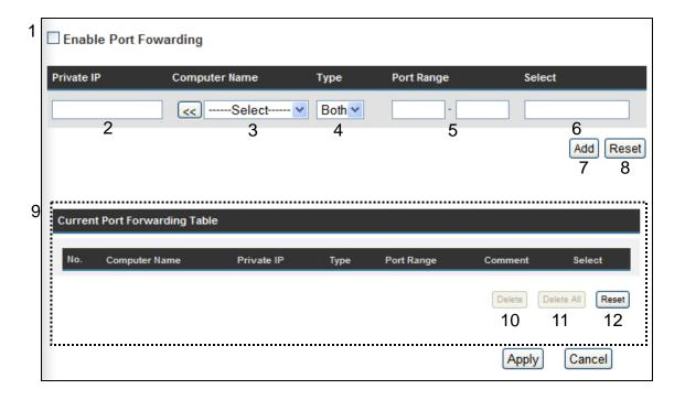
Enable Port Check this box to enable port mapping,
