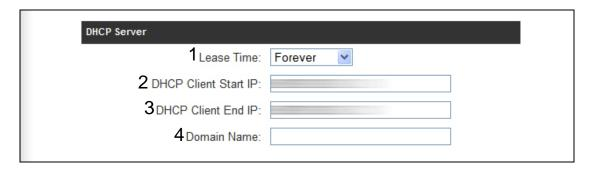
These settings are only available when 'DHCP Server' in 'LAN IP' section is "Enabled".
