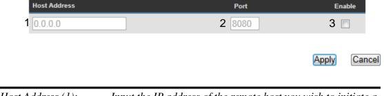
Host Address (1): Input the IP address of the remote host you wish to initiate a management access.
