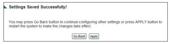
Press "Go Back" to save the settings and go back to the web management interface; press "Apply" to save the settings made and restart the Smart Dish Repeater. The settings will take effect after it reboots.
