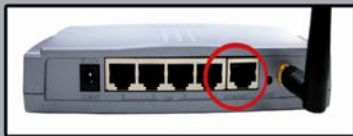
INTERNET or WAN Port on the Router Note* The WAN port on Routers may vary from different brands. If you are not sure the location or name the one on your router, check the users manual.
