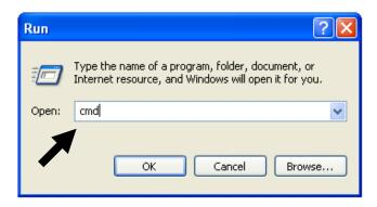
Input 'ipconfig', then press 'Enter' key. Please check the IP address followed by 'Default Gateway' (In this example, the IP address of Smart Repeater is 192.168.1.200, please note that this value may be different.)
