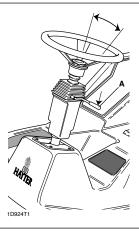
**Adjusting the length of the steering column:** Move the lever 'A' upwards to adjust the length of the steering column. Release the lever to lock the steering column in position.
