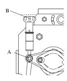
Tighten nut 'A' both ends.
