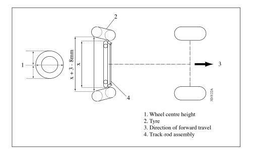
To adjust the alignment of the rear wheels, first back off the left hand and right hand locknuts on the track rod assembly. (Left hand locknut is a left hand thread). Rotate the track rod to achieve the correct 'toe - in' as described above and tighten the locknuts securely.
