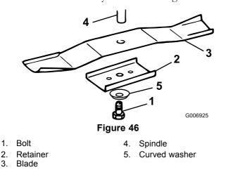
4. Inspect all parts; replace any parts that are damaged.
