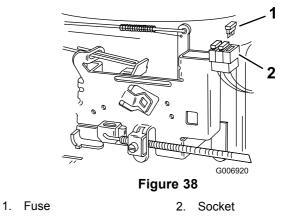
2. Insert the fuse into socket and push down on the fuse to install it.
