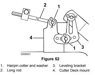
10. Remove the hairpin cotter and washer at the cutter deck leveling bracket (Figure 52). Slide the bracket
