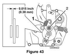
1. Brake arm spring 2. Brake adjusting nut
