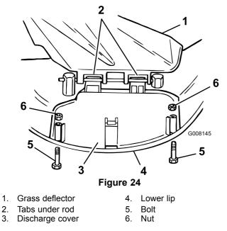
4. Secure the discharge cover to the lower lip of the cutter deck with bolts and nuts (Figure 24).
