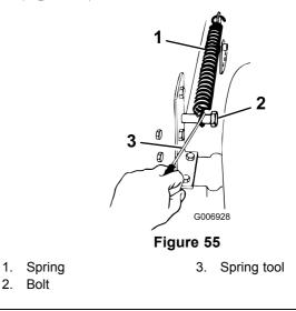
**Note:** Use the spring tool provided with the machine.
