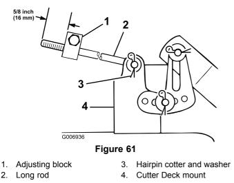
7. Install the end of the rod into the hole in the cutter deck mount and secure it with the washer and hairpin cotter.
