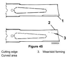
Inspect the blades, especially the curved area (Figure 45). If you notice any damage, wear, or a slot forming in this area (Figure 45), immediately install a
