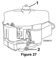
1. Oil dipstick/fill hole 2. Oil drain plug
