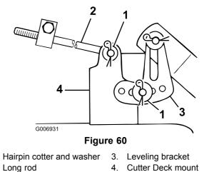
8. Position the leveling bracket in a different hole and install the washer and hairpin cotter (Figure 60).
