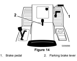
2. Lift the parking brake lever (Figure 14) up and gradually take your foot off of the brake pedal.
