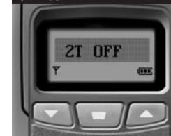
This function transmits a 2TONE signal whenever the PTT button is pressed. Select the 2TONE ANI function by pressing the "Function" button 6 times, the icon "2T" will begin flashing. Select On/Off by pressing the Up/Down buttons. The selected function will be stored automatically. If no buttons are pressed within 5 seconds after selecting functions, the
