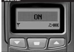
This function confirms that the buttons are properly pressed with the beep sound. Press the "Function" button 3 times to select the beep sound. The icon "♪" will be flashing. Select On/Off by pressing the Up/Down buttons. The selected function will be stored automatically. If no buttons are pressed within 5 seconds after selecting functions, the monitor will revert to the main display. Press the PTT button to finish and exit the function mode.
