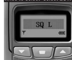
This is a sensitivity adjustment function that allows for communication at a desired level. Press the "Function" button twice to select Squelch system. The icon " **SQ** " will begin flashing. Select Low/High by pressing the Up/Down buttons. The selected function will be stored automatically. If no buttons are pressed within 5 seconds after selecting functions, the monitor will revert to the main display. Press the PTT button to finish and exit the function mode.
