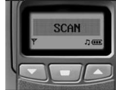
This function helps automatically find all channels used by the radio. Select the Channel Scan by pressing the "Function" button once.
