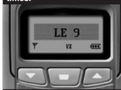
This function selects the desired sensitivity (9 Levels) to activate the VOX circuit. Select the VOX Mode by pressing the "Function" button 8 times. The icon "LE" will begin flashing. Select the VOX level desired by pressing the Up/Down buttons. Pressing the PTT button saves the selected level and exits the function mode.
