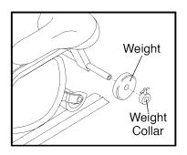
the desired amount of weight onto the weight bar and reattach the weight collars. Note: Place equal amounts of weight on both sides of the weight bar. The combined weight of the user and added weights should not exceed 300 pounds.
