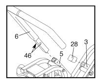
and slide the Handlebar Assembly (6) out of the Handlebar Swing Arm (5). Press the Snap Buttons again and insert the Handlebar Assembly into the Wheel Swing Arm (3). **Make sure that the Snap Buttons snap into the holes in the Wheel Swing Arm.** Press the Swing Arm Cap (28) onto the Handlebar Swing Arm (5).
