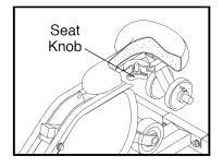
adjusted, sit on the seat and pull the handlebar as close as possible to your stomach. Your legs should be almost straight, with your knees bent slightly.
