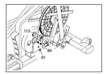
Reattach the right shield, the right roller arm, the right pedal arm, the shield cover cap, and the shield cover.
