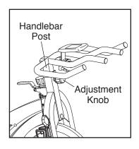
Make sure that the adjustment knob is engaged in an adjustment hole.
