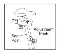
the adjustment knob. Make sure that the adjustment knob is engaged in an adjustment hole.
