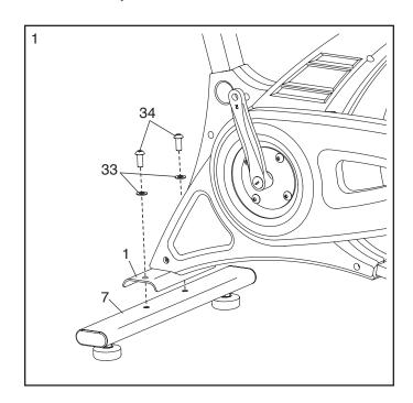
Remove the two screws, the two washers, and the shipping bracket (not shown) from the front of the Frame (1). Discard the screws, washers, and shipping bracket.
