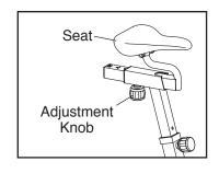
hole in the seat carriage, and firmly tighten the adjustment knob. Make sure that the adjustment knob is engaged in an adjustment hole.
