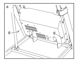
Lower the treadmill (see HOW TO LOWER THE TREADMILL FOR USE on page 22). Remove the three #8 x 3/4" Screws (6). Carefully slide the Motor Hood (57) off.
