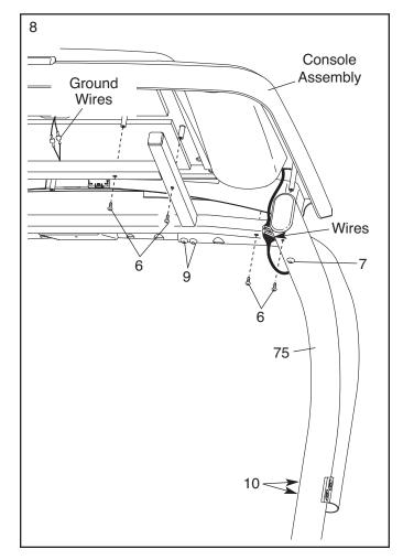
Attach the Pulse Bar Bottom (90) to the console assembly with six #8 x 3/4" Screws (6); start all six Screws, and then tighten each of them. Do not overtighten the Screws.
