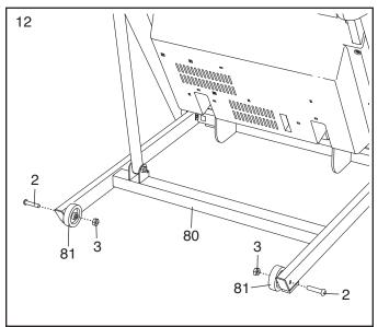
13. **Make sure that all parts are properly tightened before you use the treadmill.** If there are sheets of plastic on the treadmill decals, remove the plastic. To protect the floor or carpet, place a mat under the treadmill. Note: Extra hardware may be included. Keep the included hex key in a secure place; the hex key is used to adjust the walking belt (see pages 24 and 25).
