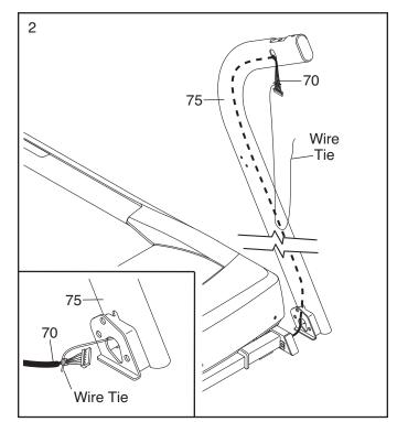
Hold the Left Upright (75) against the Base (80). Be careful not to pinch the wires. Insert a 3/8" x 4" Patch Bolt (4) with a 3/8" Star Washer (5) into the top hole in the Left Upright.
